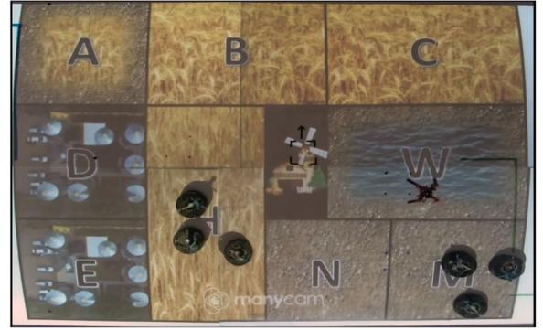
Fig. 7. Overhead view of Demonstration 2. Note 6 ground robots and 1 aerial robot. Two ground robots have camera and small harvester capabilities (one in H and one in M), the 4 other ground robots have the large harvester and small harvester capabilities, and the drone has only the camera capability.
