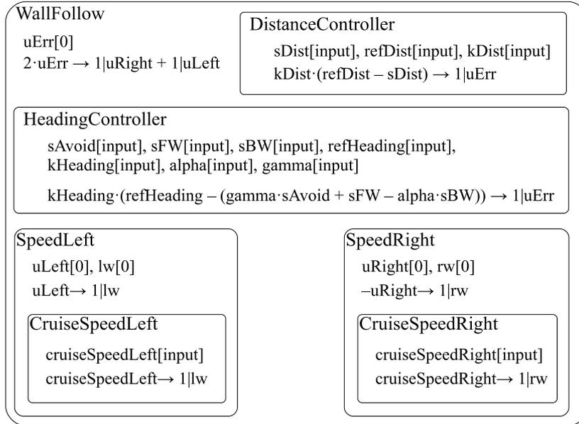
Figure 8: Membrane controller for the wall following behaviour
