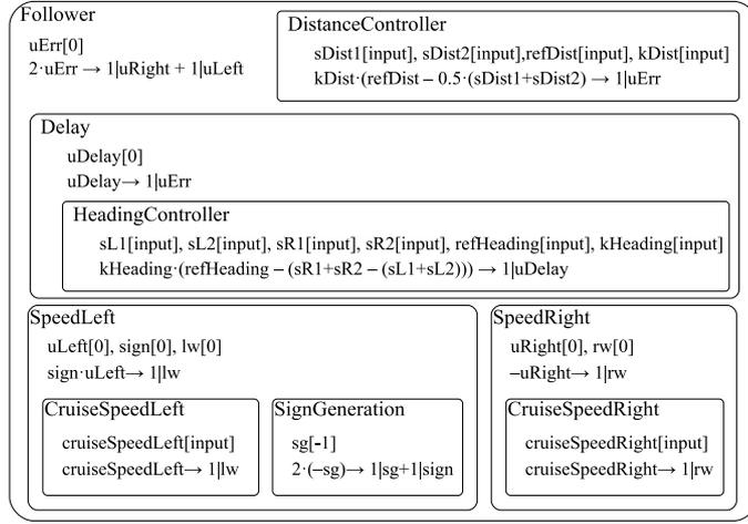
Figure 9: Membrane controller for the follower behaviour
