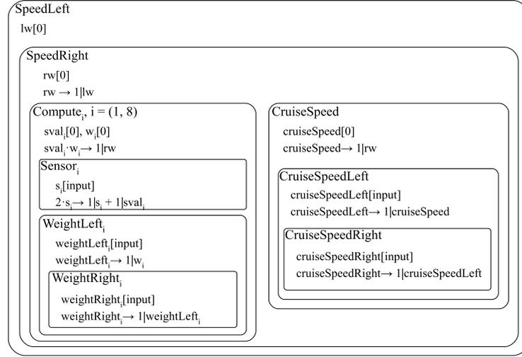
Figure 7: Membrane controller for the obstacle avoidance behaviour
