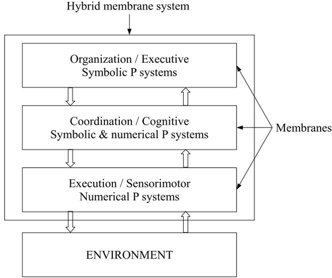
Figure 5: Cognitive architectures as hybrid membrane systems
