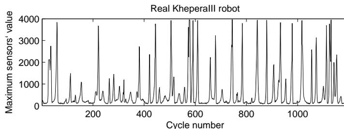
Figure 16: Performance indices in each cycle for the Khepera III robot with fuzzy controller for obstacle avoidance
