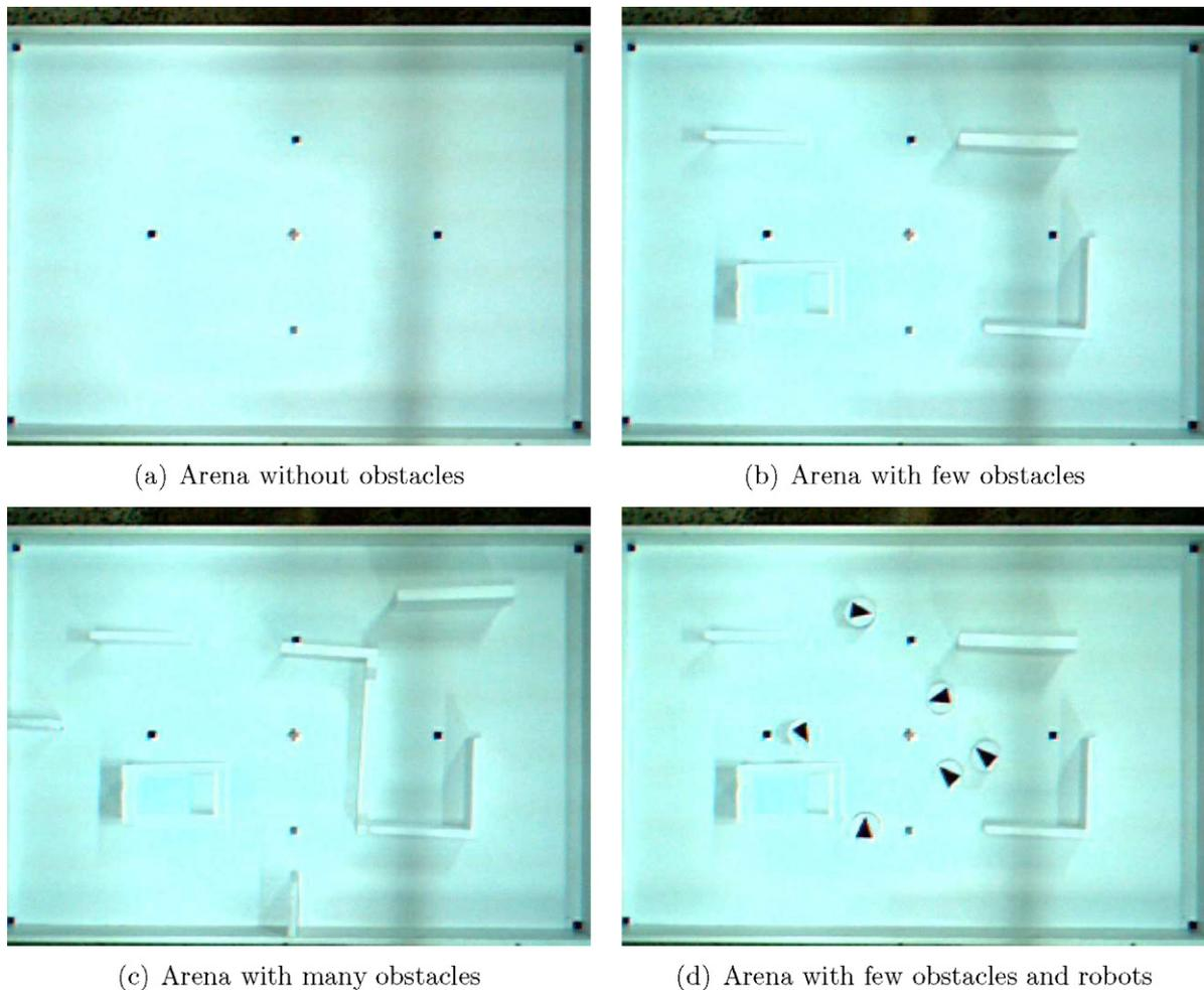
**Fig. 6.** Arena configuration for the e-puck experiments. (a) Arena without obstacles, (b) arena with few obstacles, (c) arena with many obstacles and (d) arena with few obstacles and robots.
