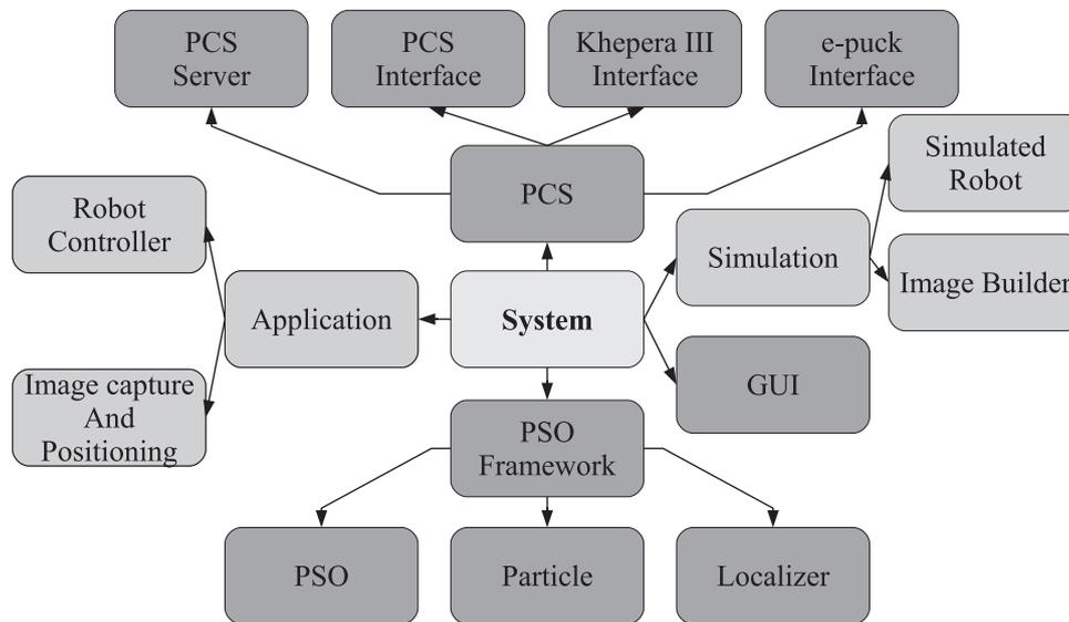
Fig. 1. Block diagram of the software system.
