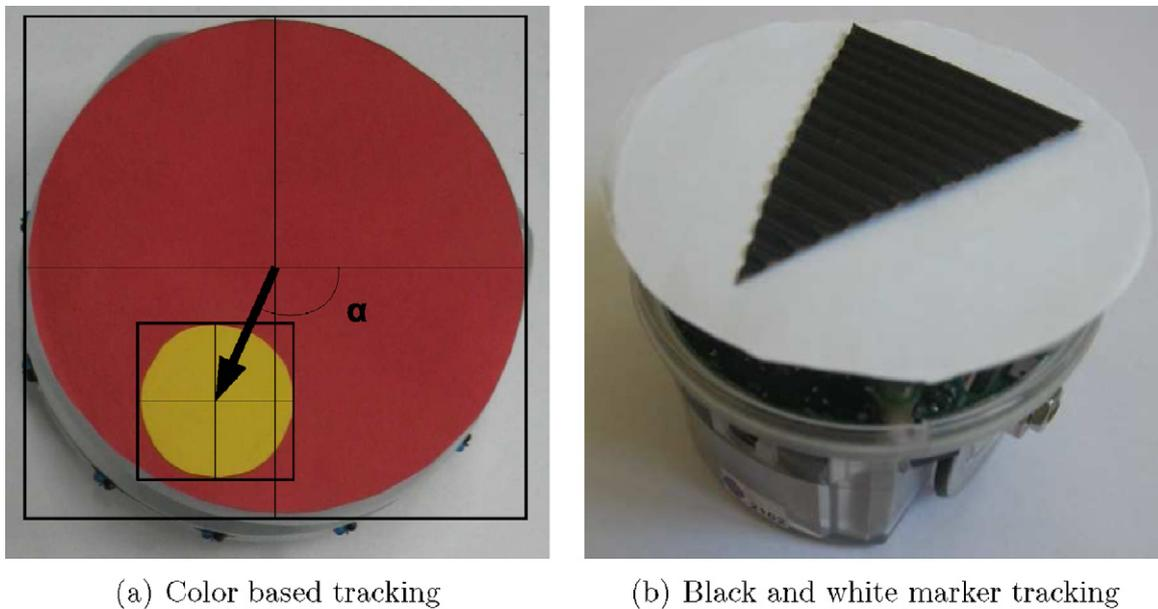
Fig. 5. Robot localization. (a) Color based tracking and (b) black and white marker tracking.
