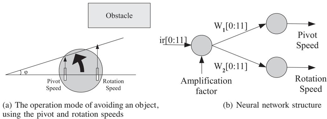
**Fig. 4.** Obstacle avoidance behaviour. (a) The operation mode of avoiding an object, using the pivot and rotation speeds and (b) neural network structure.
