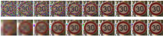
(a) Example images with: 1) Fixed relative resolution (100%) with various noise levels; 2) Fixed noise level b_t = 0.04 with various resolution levels;
